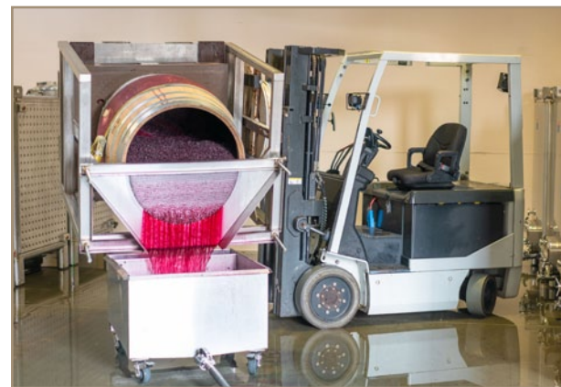
Luc designed the Gyrobox™ to drain puncheons by gravity
