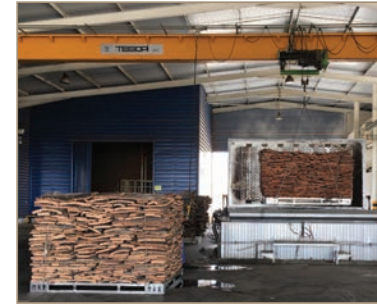
The pallet of planks on the right is being raised out of M. A. Silva's Dynavox® cleansing system.
