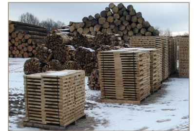
Staves are exposed to the elements, Méry-ès-bois, France
