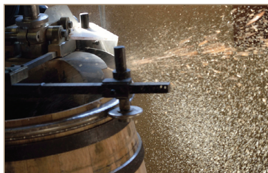
A croze cuts the grooves needed to attach the heads of the barrel, Tonnellerie Darnajou
