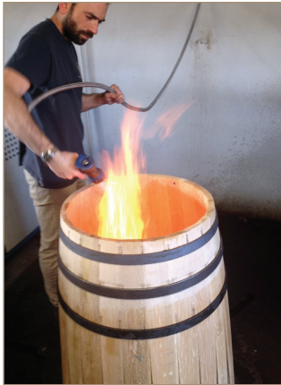
Vincent Darnajou uses fire and water to give a barrel its shape
