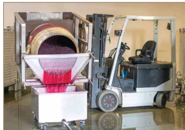
The Gyrobox™ which Luc designed drains a puncheon after fermentation and maceration are completed
